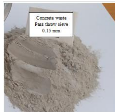
Figure 3. The sample of Concrete Waste
